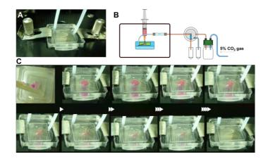
**Supplementary Figure 4.** Testing the efficiency of pressure-driven medium change in cell culture system. (A) Picture of the cell culture system after assembly. (B) Schematic of a microchip-based device. (C) Photograph showing liquid change process.
