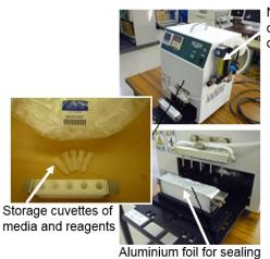
N<sub>2</sub> gas flowmeter for oxidization prevention of the culture media/reagents
