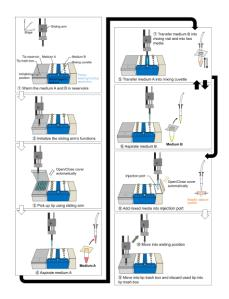
**Supplementary Figure 6.** Schematic showing how the robotic arm for liquid handling supply culture medium in chip.
